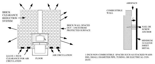
BRICK WALLS MAY BE ATTACHED TO COMBUSTIBLE WALLS USING WALL TIES. IF BRICK IS USED, BE SURE FLOOR CAN WITHSTAND THE WEIGHT OF THE BRICK.
