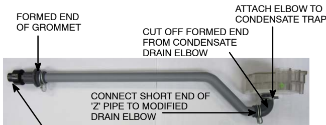
Figure 17 – Accessory Horizontal Drain Trap Grommet
