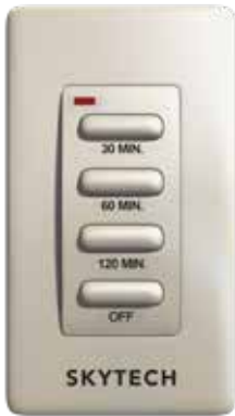
TM-R-AF1TX TFS Wireless Wall Timer (30min/60min/120min), twenty (20) foot range, surface mount, battery operated, uses two 3-volt button cell batteries (included) - (TFS units only)
