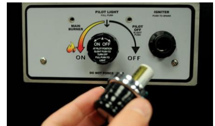
Figure 10.5 – Remove igniter unit cap with battery.
