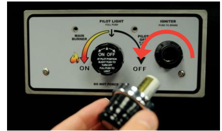
Figure 10.4 – Unscrew spark igniter unit cap.
