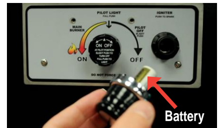
Figure 10.6 – Slide battery into spark igniter unit.
