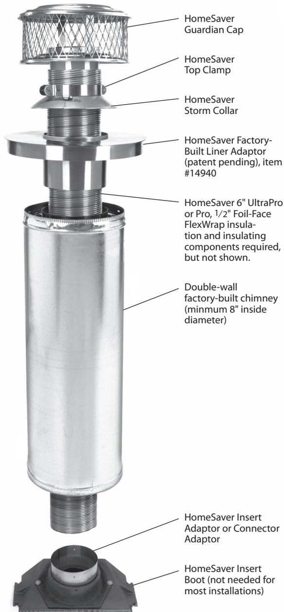
**FIGURE 14 – COMPONENTS OF A FACTORY BUILT CHIMNEY RELINE**
