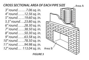
proper draft. If the chimney is offset, or if the liner is square, oval or rectangular, the flue liner shall not be less than  $\frac{1}{10}$  of the fireplace opening. You should refer to the current NFPA 211 for additional sizing specifications.
