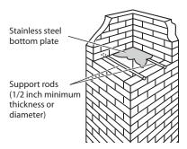
FIGURE 11 - LINER SUPPORT RODS
