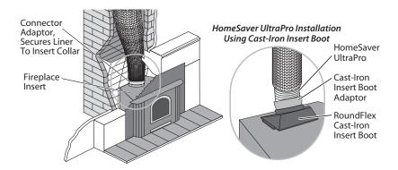
FIGURE 8 - LINER CONNECTION TO FIREPLACE INSERT
