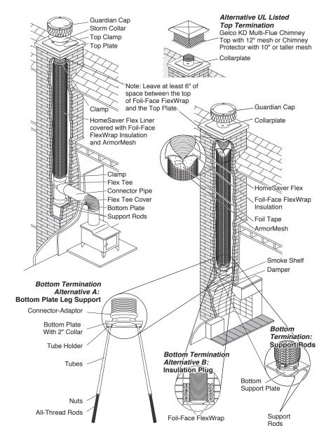
FIGURE 12 - ALTERNATIVE TOP AND BOTTOM INSTALLATIONS
