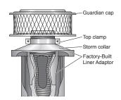
FIGURE 6 – TOP OF FACTORY-BUILT CHIMNEY INSTALLATION
