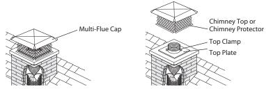
FIGURE 15 - COVER TOP TERMINATION WITH CHIMNEY CAP
