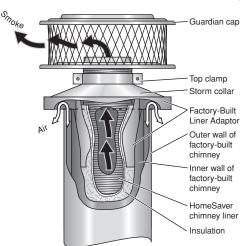
FIGURE 13 - FLOW DIAGRAM OF FBLA ADAPTOR
