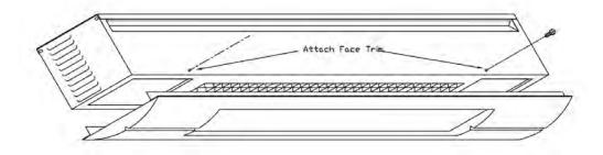
Optional Face Trim can be easily installed on all Sunpak models.
