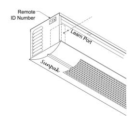
The Sunpak S34-TSR should <u>always</u> be started up and operated on the HIGH mode for the first 5 minutes to allow the heater to warm up. Starting up the heater on the LOW mode before the heater is warmed up may cause the heater to shut down prematurely. To correct this situation press the OFF button followed by the ON button and the HI button. Always PRESS the button for at least 1 second to allow proper transmission of the remote signal.
