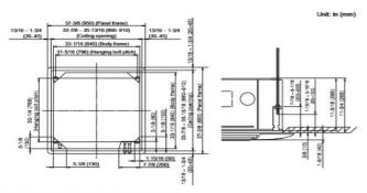
Refrigerant piping and drain piping positions
