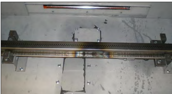
STEP 1: Remove false bottom to expose burner tube. Remove burner tube and cover plate as above. Remove old sealant from opening.
