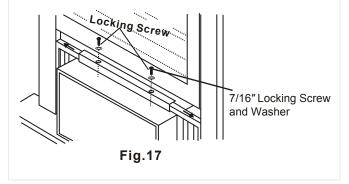
4. Attach the top angle to window frame: Use a 3/32" drill bit to drill one hole through the hole in the middle of top angle into the window frame, and drive one 3/4" (or 1/2") HEX-HEAD locking screw through hole in the middle of top angle into the window frame as shown (Fig. 17A).
