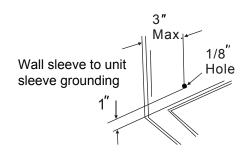
4. Prepare the wall sleeve for installation of the new unit per the following brand instructions:
