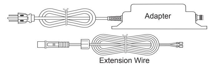
**Description:** This is an outdoor approved adapter suited for wet, damp dry locations. It plugs into 120VAC outlet and converts it to 6-volts DC to operate Firegear Outdoor electronic systems. Each model comes with an adapter and 5-foot power cord. The ADP10-OUT includes the adapter and a 10-foot extension wire. The ADP70-OUT includes the adapter and a 70-foot extension wire.
