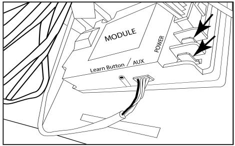
**Fig. 2** Shows location of control module's two ½" terminals (labeled POWER) to attach adapter.
