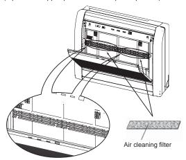
3. Install the Air filter and close the Intake Grille.
