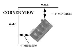
NOTE: TYPICAL STOVE CABINET MODEL FIGURE 6 - MINIMUM CLEARANCES TO WALLS AND CEILING
