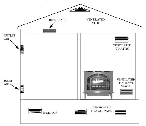
FIGURE 3 - VENTILATION AIR FROM OUTDOORS
