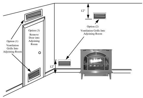
FIGURE 2 - VENTILATION AIR FROM INSIDE BUILDING
