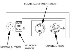
FIGURE 16 - CONTROL KNOB AND IGNITOR BUTTON LOCATION
