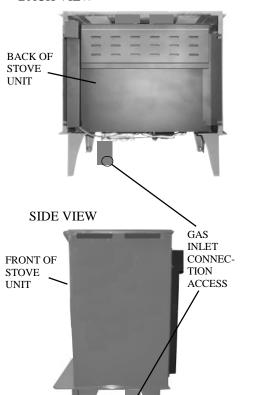
Installation must include an equipment shutoff valve, union and plugged 1/8" NPT tap. Locate NPT tap within reach for test gauge hook up. NPT tap must be upstream from heater (See Figure 8).
