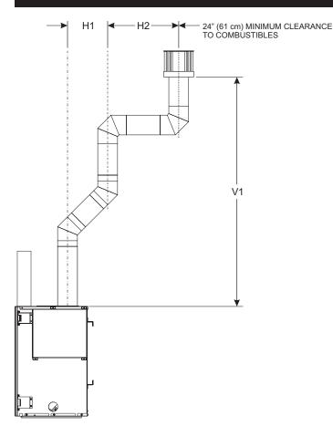
If total horizontal needs to be 8' (2.44 m), then the minimum required vertical is 5' (1.52 m).
