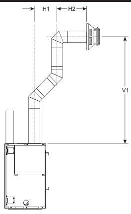
If total vertical is to be 9' (2.74 m), then the maximum allowed horizontal run can be 20' (6.10 m).
