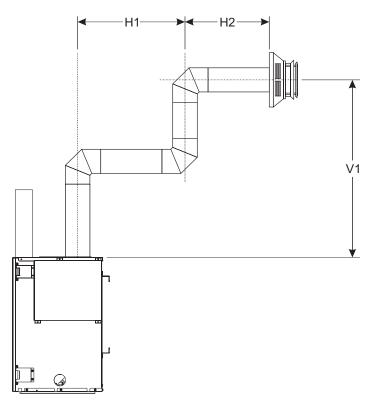
If total horizontal needs to be 10 $^{\circ}$  (3.05 m), then the minimum required vertical is 7 $^{\circ}$  (2.13 m).
