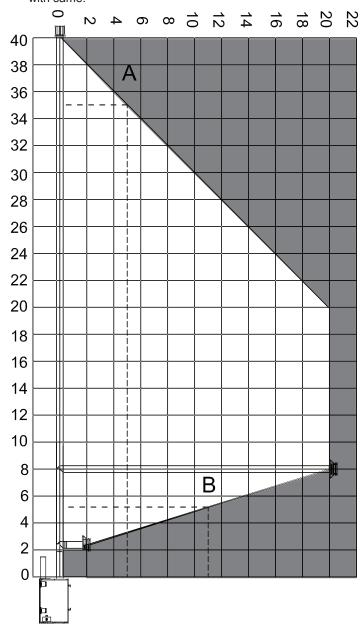
Acceptable vertical and horizontal vent run. (40 ft. (12.19 m) maximum vertical and 20 ft. (6.10 m) maximum horizontal)
