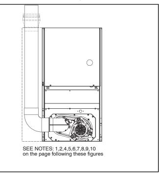
Figure 40 – Downflow Application–Vent Elbow Up then Right
