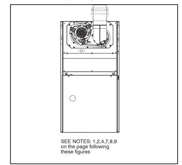
Figure 36 – Upflow Application–Vent Elbow Right
