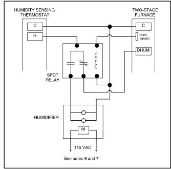
Figure 32 – HP with Two–Stage Furnace, Humidifier, and Dehumidification
