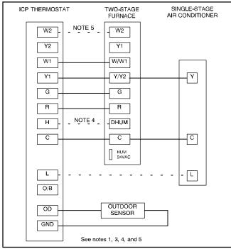
Figure 27 – Two-Stage Furnace with Two-Stage Air Conditioner
