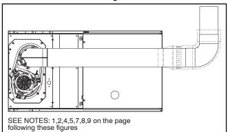
A03216 Figure 46 – Horizontal Right Application – Vent Elbow Left then Up
