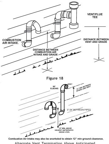
Combustion Air Intake may also be snorkeled to obtain 12" min ground clearanc Alternate Vent Termination Above Anticipated Snow Level (Dual Pipe) Figure 19
