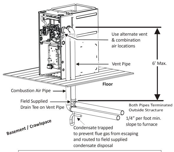
All piping and fittings must be joined per material manufacturers specifications to prevent separation and flue gas leaks.
