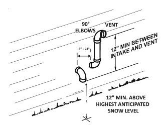
Alternate Horizontal Vent Termination (Dual Pipe) Figure 17
