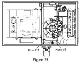
1. Remove the clamps from both ends of the drain hoses.
