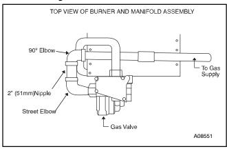
Figure 22 - Typical Gas Pipe Arrangement
