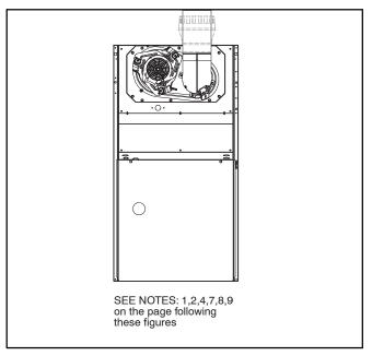
Figure 29 — Upflow Application-Vent Elbow Right
