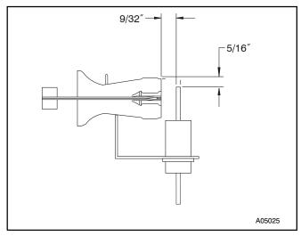
Figure 46 - Igniter Position-Top View
