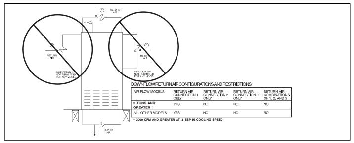
Figure 20 — Horizontal Return Air Configurations and Restrictions
