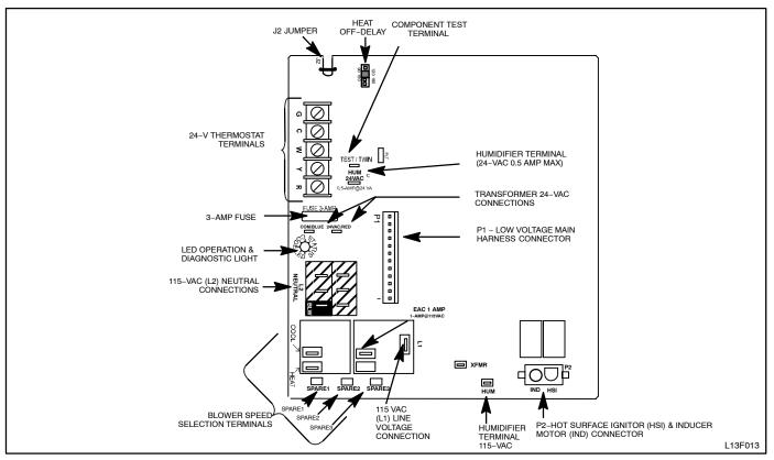
Figure 26 — Heating and Cooling Application Wiring Diagram with Single Stage Thermostat
