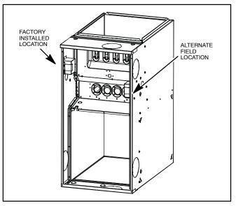
Figure 24 — Field-Supplied Electrical Box on Furnace
