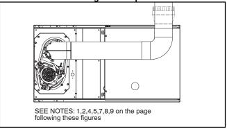
Figure 36 — Horizontal Left Application-Vent Elbow Up
