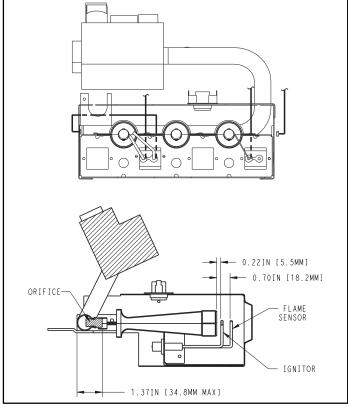
Figure 4 - Two-Stage Igniter, Flame Sensor, Orifice/Main **Burner Relationship**
