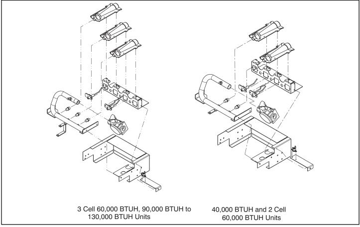
Figure 15 - Single-Stage Orifice Installation
