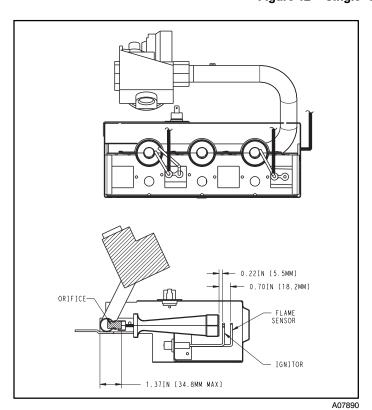
Figure 13 - Single-Stage Igniter, Flame Sensor, Orifice/Main Burner Relationship
