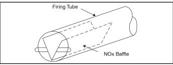
Figure 1 - Low NOx Baffle Location
