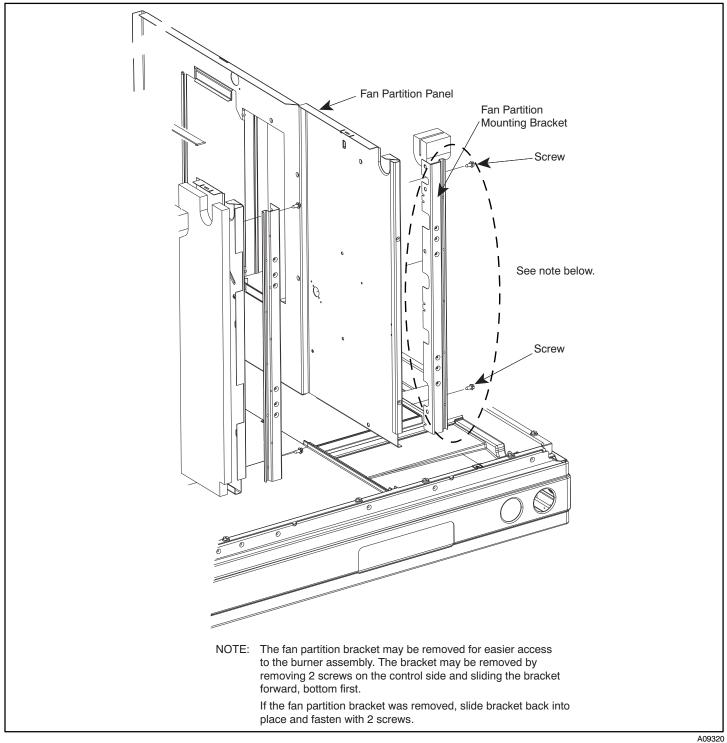
Figure 2 - Fan Partition Bracket Removal
