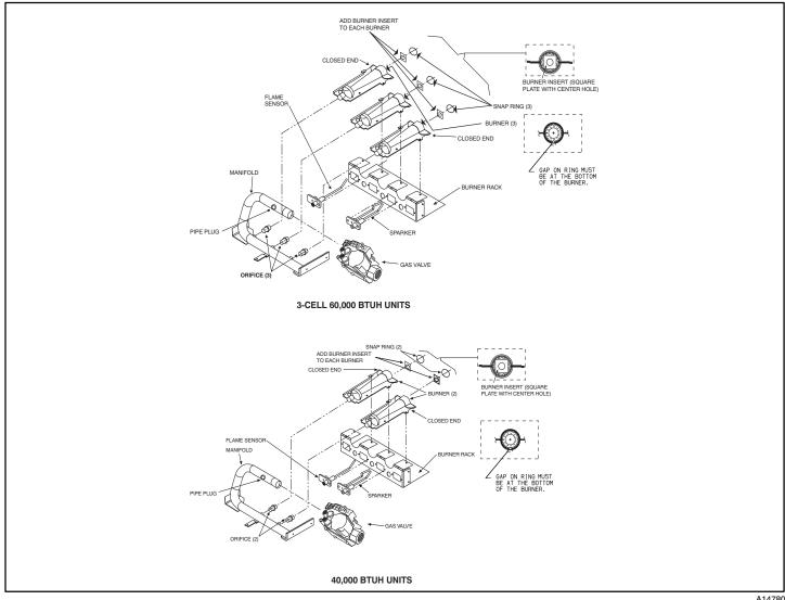
Figure 7 - Orifice and Burner Insert Installation
