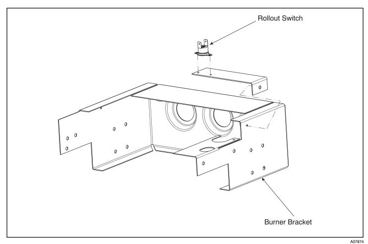
Figure 12 - Single-Stage Burner Bracket
