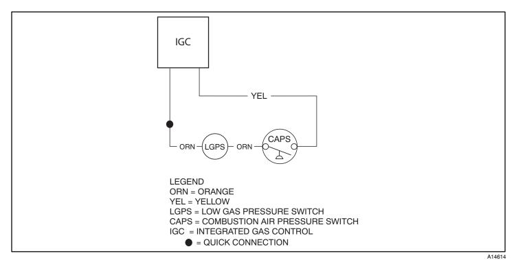
Figure 8 - Pressure Switch Wiring
