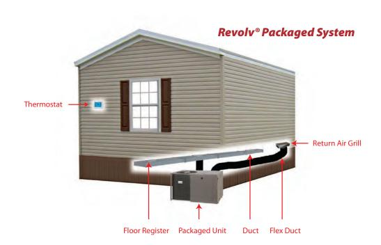
**Revolv Packaged System** – Packaged units provide both heating and cooling from one unit that is placed outside the home. Packaged units are available in several combinations of fuel sources - gas heat/electric cooling; heat pump and electric heat/electric cooling.
