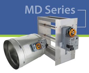
The MD Series dampers are perfect for use with most zoning systems and recommended for use with our ESP zone panels. These dampers are shipped complete and ready for installation. The MD Series dampers can be installed in any position. They are rated for duct systems less than 1.0" WC. The MD Series dampers have a simple adjustment for setting the minimum position.
