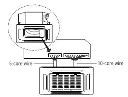
Fasten the control box lid with 2 screws.
