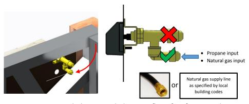
2. Lay the burner upside down on a flat, soft surface to avoid scratching the polished metal. Ensure the correct orifice is installed for the fuel type you are using (see Crystal Fire user manual included with burner for orifice sizing information) Attach the included metal flex hose to the burner.
