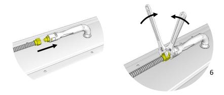
3. Set the burner into the fire pit table exactly as shown and make final gas connection to the control panel.
