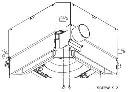
\* When using the "UTZ-KXGC" kit for high humidity, please first cut off and remove the heat insulation as shown in the figure.
