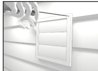
**3** Push the hood into the opening and then attach the hood to the outside wall with mounting screws. Repeat the installation procedure for both the supply and exhaust hoods.
