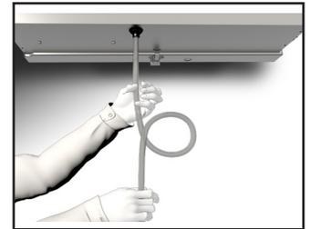
**4** Install the drain hose making a "P" trap, secure the condensate line drain connection using the tube clamp provided. Fill the condensate line with water.
