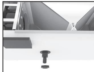
**3** Secure the drain nipple using the nutsert.
