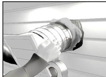
**2** Pull the insulated flexible duct through the opening until it is well extended and straight. Slide the duct's inner vinyl sleeve over the hood duct connection and secure. Pull the insulation over the duct and pull the vapor barrier over the sleeve. Secure with appropriate tape or sealant.
