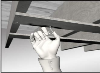
**1** Place fastening hooks on the strapping board or the floor joists.
