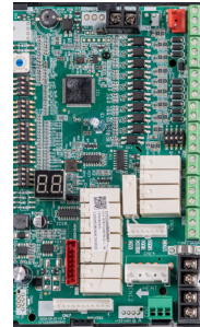
INDOOR AHU CONTROL BOARD
