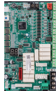
INDOOR AHU CONTROL BOARD
