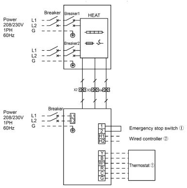
Note: ①The factory has been short-circuited, when the user needs to connect the emergency stop switch, please remove the corresponding short-circuit wire
