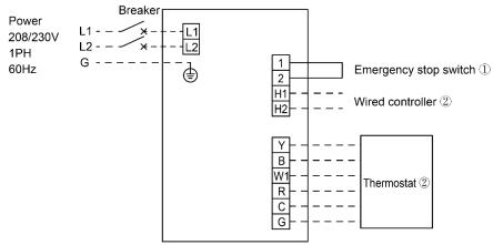
Note: ①The factory has been short-circuited, when the user needs to connect the emergency stop switch, please remove the corresponding short-circuit wire
