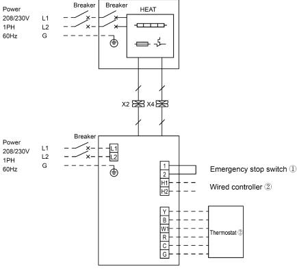
Note: ①The factory has been short-circuited, when the user needs to connect the emergency stop switch, please remove the corresponding short-circuit wire
