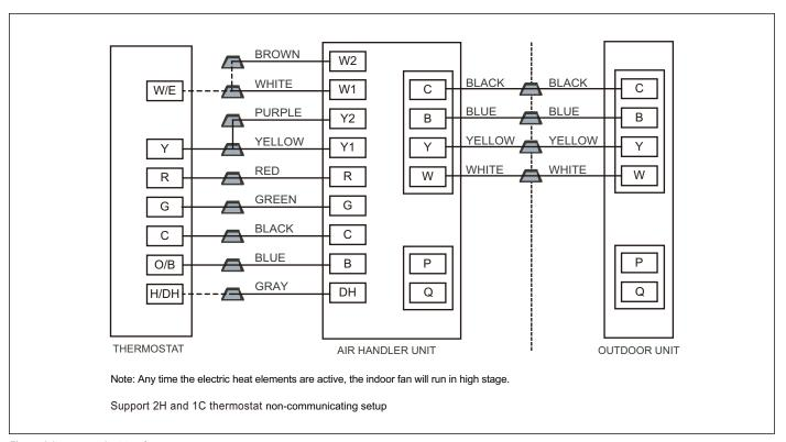
Figure 34 Control wiring for HP systems
