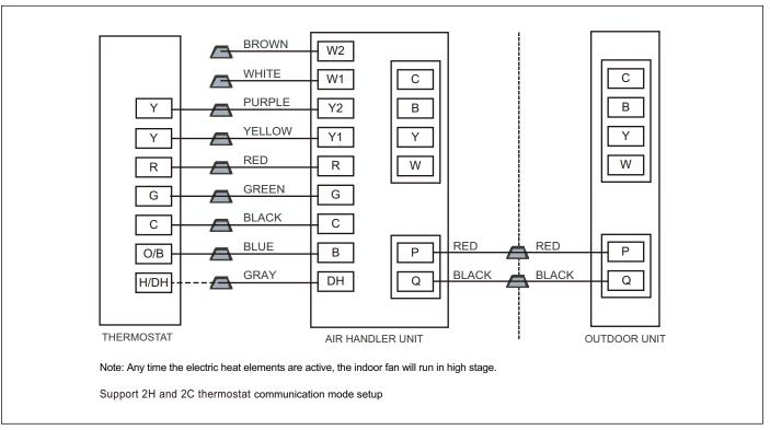
Figure 43 Control wiring for HP systems
