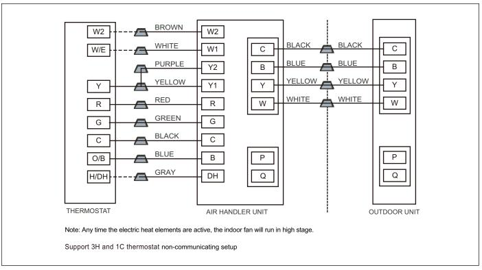
Figure 31 Control wiring for HP systems
