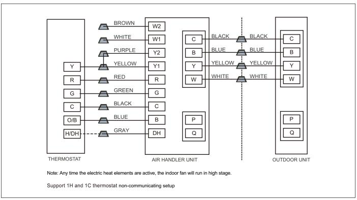
Figure 33 Control wiring for HP systems
