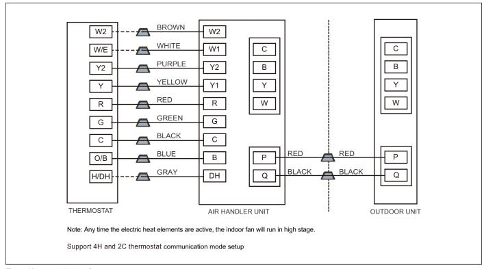
Figure 41 Control wiring for HP systems
