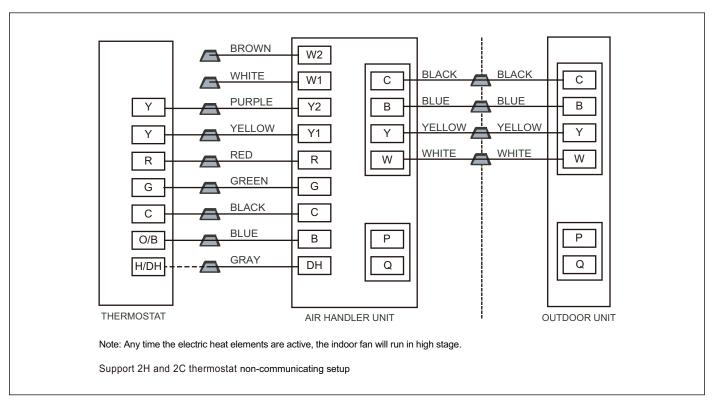
Figure 32 Control wiring for HP systems
