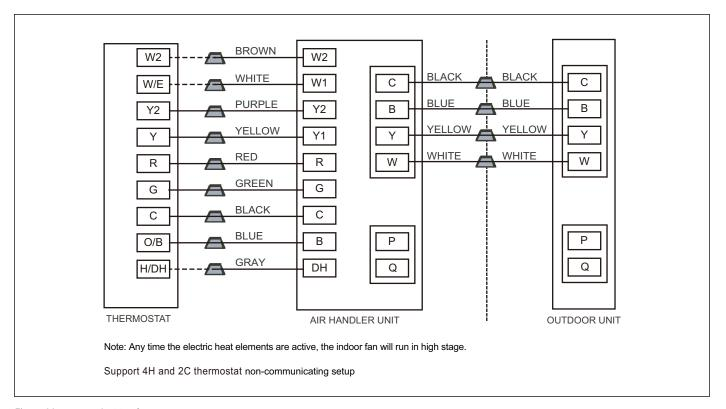
Figure 30 Control wiring for HP systems
