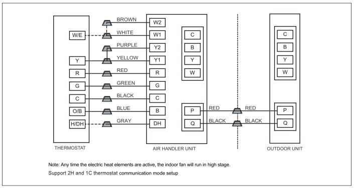
Figure 46 Control wiring for HP systems
