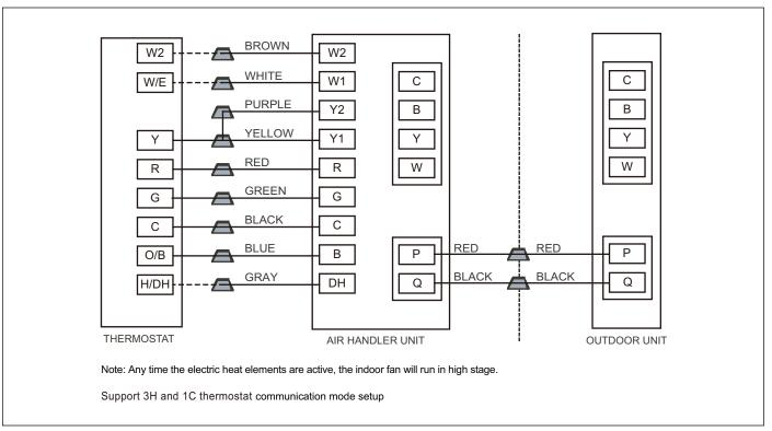
Figure 42 Control wiring for HP systems
