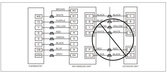
Figure 47 Incorrect wiring example
