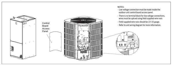
Figure 26 Low Voltage Unit Connections
