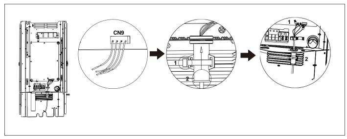
Figure 28 Wires connections diagram
