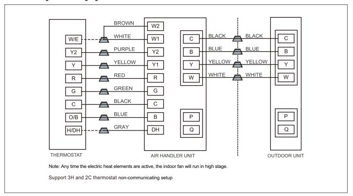
Figure 29 Control wiring for HP systems
