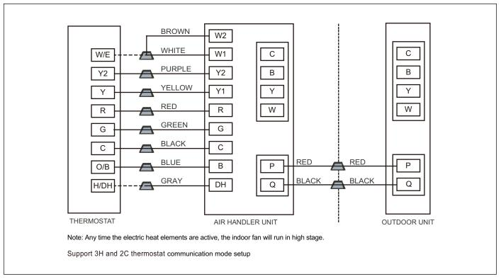
Figure 40 Control wiring for HP systems
