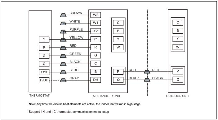
Figure 45 Control wiring for HP systems
