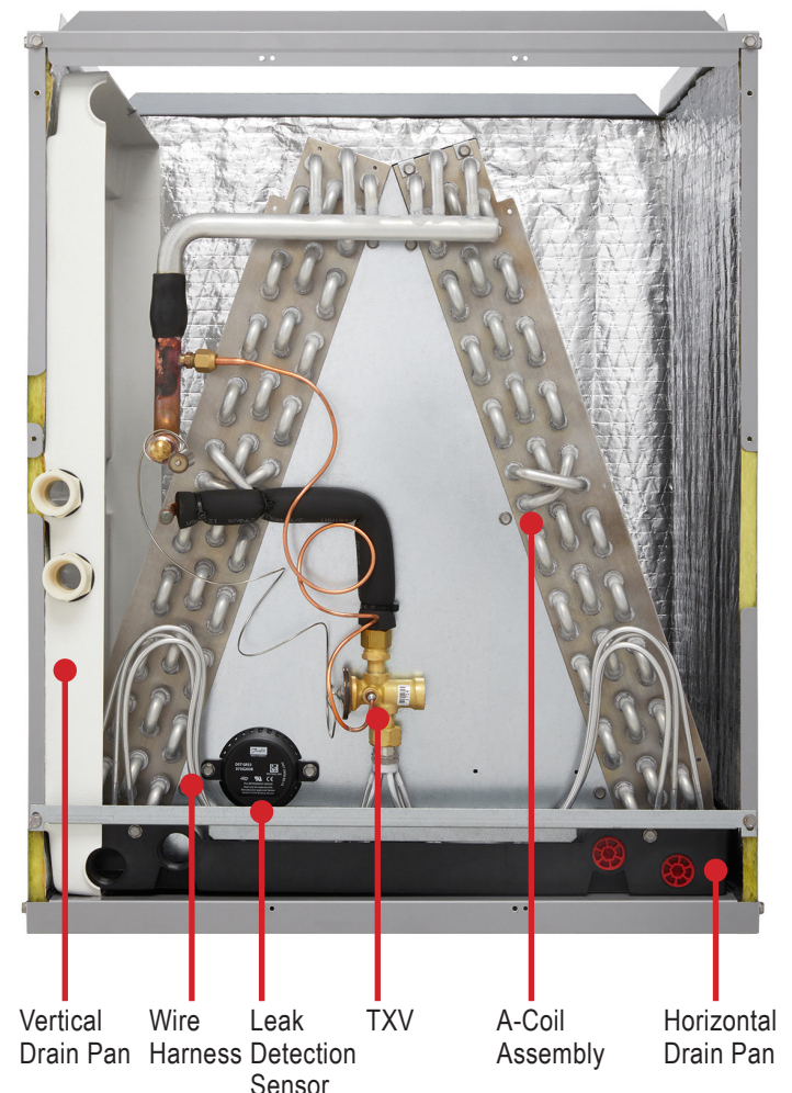
Figure 3: A-Coil Components.
