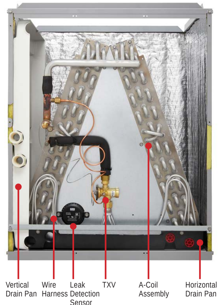
Figure 3: A-Coil Components.
