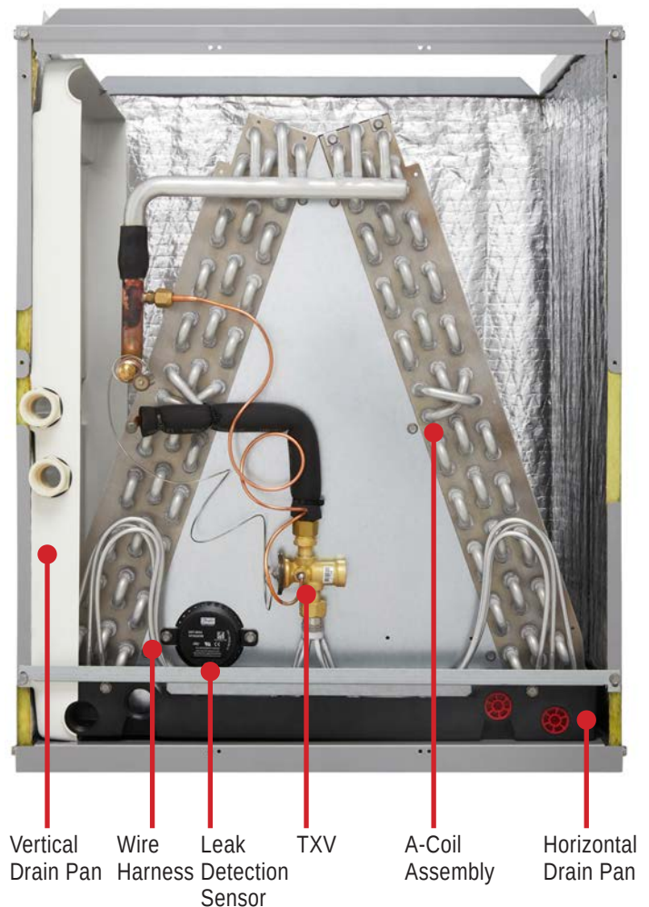
Figure 3: A-Coil Components.
