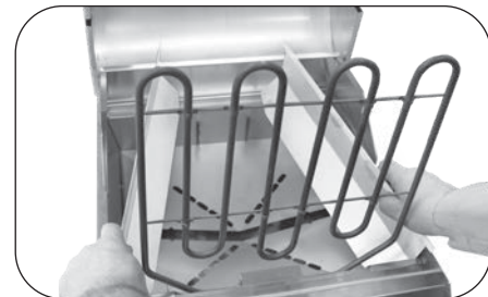
Fig. 22-3 Remove side liners
