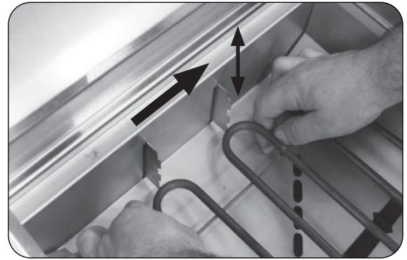
Fig. 18-1 Adjust cooking element
