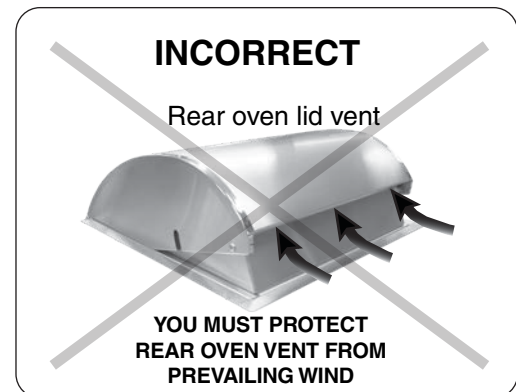
Fig. 8-3 Airflow direction - INCORRECT
