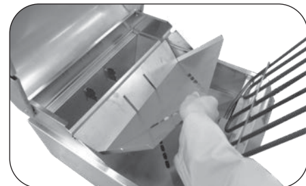
Fig. 22-4 Remove rear liner
