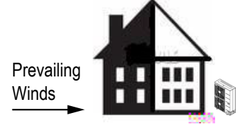
Figure 31: Leeward Side of the Building.
