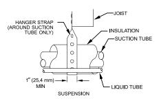
Fig. 1 – Connecting Tubing Installation
