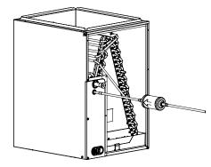
Fig. 3 – Liquid Line Filter Drier
