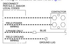
Fig. 5 – Line Power Connections
