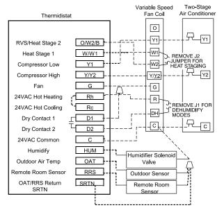
Thermidistat w/Variable Speed Fan Coil & 2-Stage Air Conditioner
