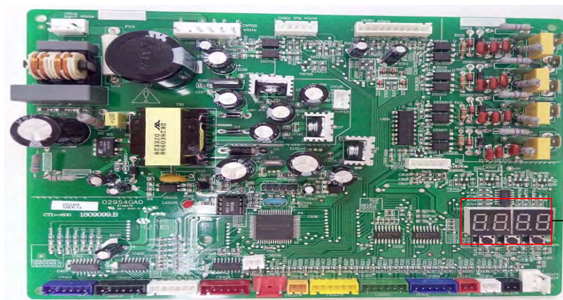
Outdoor Control Board
