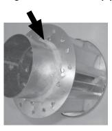
STEP 5: Before sealant can dry, insert collar on vent cap as far as possible inside inner wall of double-wall pipe. Apply silicone sealant to fully close any gaps between vent cap and double-wall pipe to prevent water from entering double-wall pipe.
