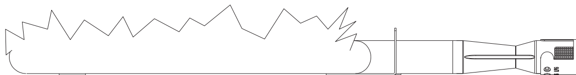
Poor Combustion: wavy, yellow flames-too little air
