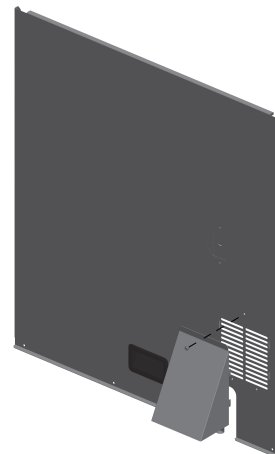
Figure 14. Vent hood installation
