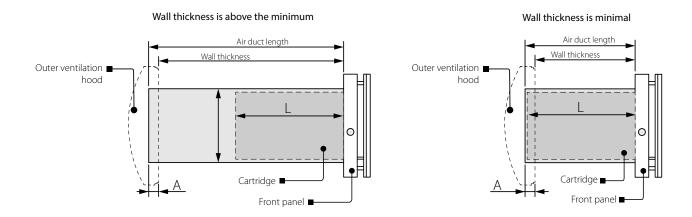
The air duct length depends on the unit model, refer to the Designation Key section, page 6.
