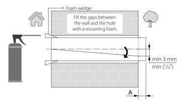
Install the air duct in the wall in such a way so it protrudes from the wall surface for maximum 3 mm or is flush with the wall. Install the air duct with the minimum slope 3 mm downwards. On the outer wall side the air duct end must protrude to a distance that enables installation of the outer ventilation hood. Distance A is stated in the installation instruction for the ventilation hood.
