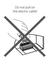
Use a flat screwdriver to disconnect the socket.
