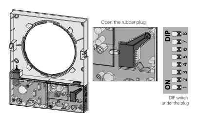
Prior to operating the ventilator set it up using the DIP switch. It is located on the controller circuit board. To access the DIP switch, take off the front panel of the indoor unit and uplift the rubber plug that covers the switch.
