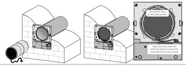
8. Install the front part of the indoor unit. The thermal actuator rod must be in lower position when installing the front panel, as shown in the figure in Section 4 on page 11.
