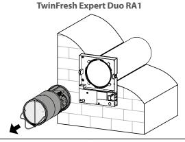
4. Wash the filters and let them dry out completely. Install the dry filters back and reassemble the unit. Vacuum cleaning is allowed. The filter rated service life is 3 years.
