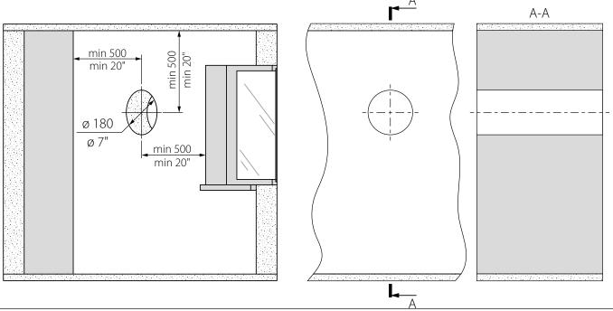
2. Install the air duct in the wall and fix it with mounting foam. The air duct end must protrude for the distance that enables installation of the outer ventilation hood (see the User's manual for the outer ventilation hood).
