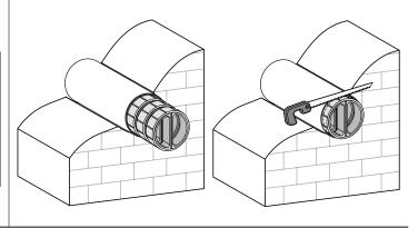
10. Install the outer ventilation hood. For this, see the user's manual for the hood.
