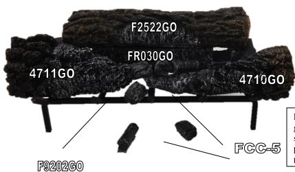
Place the FR030GO on the grate. Pull it forward until the front edge touches the front logs. This will create the heat chamber needed to help the logs glow and radiate heat.
