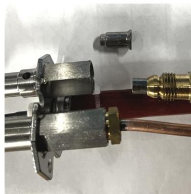
Figure 9.3 – Cleaning pilot orifice
