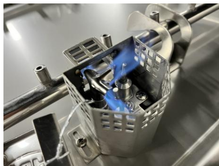
Figure 9.2 – Pilot flame coverage of thermocouple.
